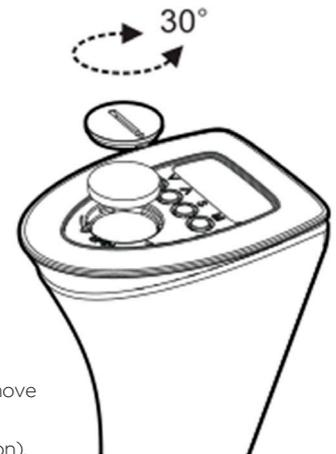
Battery replace (remove protective plastic to enable the connection).
