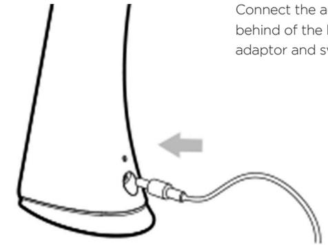
Connect the adapter in the behind of the lamp, use only adaptor and switch supplied.
